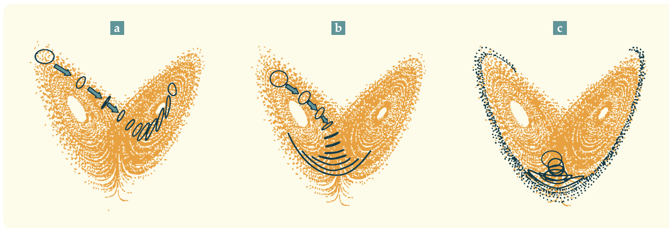
FIGURE 2. PREDICTABILITY in a nonlinear system, such as this Lorenz attractor, is dependent on the initial conditions, whose uncertainties are represented by the size and location of a circular ring. (a) The ring of uncertainty does not grow in time at all. (b) Started from a lower position, the ring distorts into banana and boomerang shapes, making it unclear whether the actual system undergoes a transition from the left-hand lobe to the right-hand one. (c) With the ring initiated almost midway between the lobes, the time evolution of the attractor is now very uncertain, and there is no predictability. (Adopted from ref. 11.)
